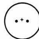
Fig 4. Combined like polarity of two close-coupled monopoles
